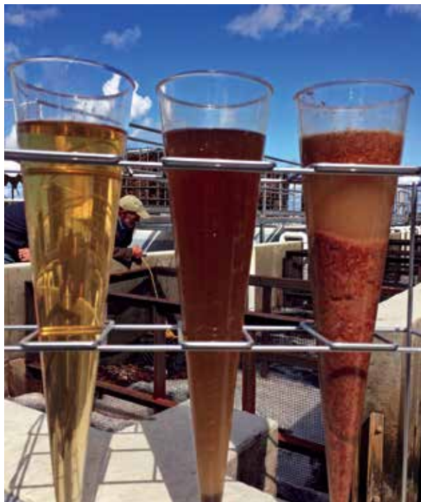
Byproducts from the distilling and brewing processes (at right) are filtered twice, passing through wood chips to replicate natural aquatic food chains (left) on a commercial scale.
